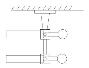
All 19mm double poles should be fitted so the pole ends within the bracket (before grub screw).
