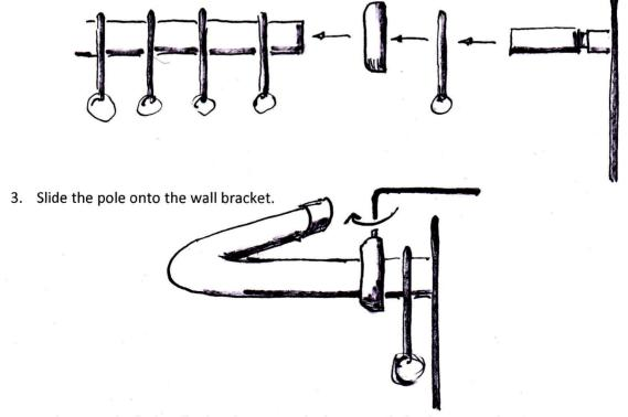
4. Tighten up the lock collar hex key using the key provided. The screw should go through the hole in the pole and lock into the wall bracket
